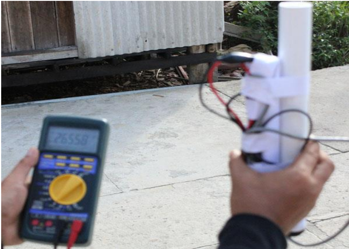
Figure 2. Measurements of solar irradiation at Air Sena using Environdata (model SR10/11) pyranometer (EnReach 2014)
