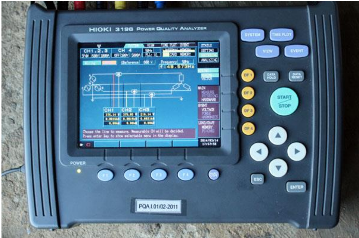
Figure III-3. Hioki 3196 Power Quality Analyser
